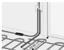
The floor temperature sensor cable has to be placed into a **separate conduit** according to EN 61386-1. It should be placed at heating level directly underneath the heating mat by chiselling out a channel in the subfloor. The sensor should be centrally positioned between two heating conductors, which is in the middle of a cable loop. Route the
